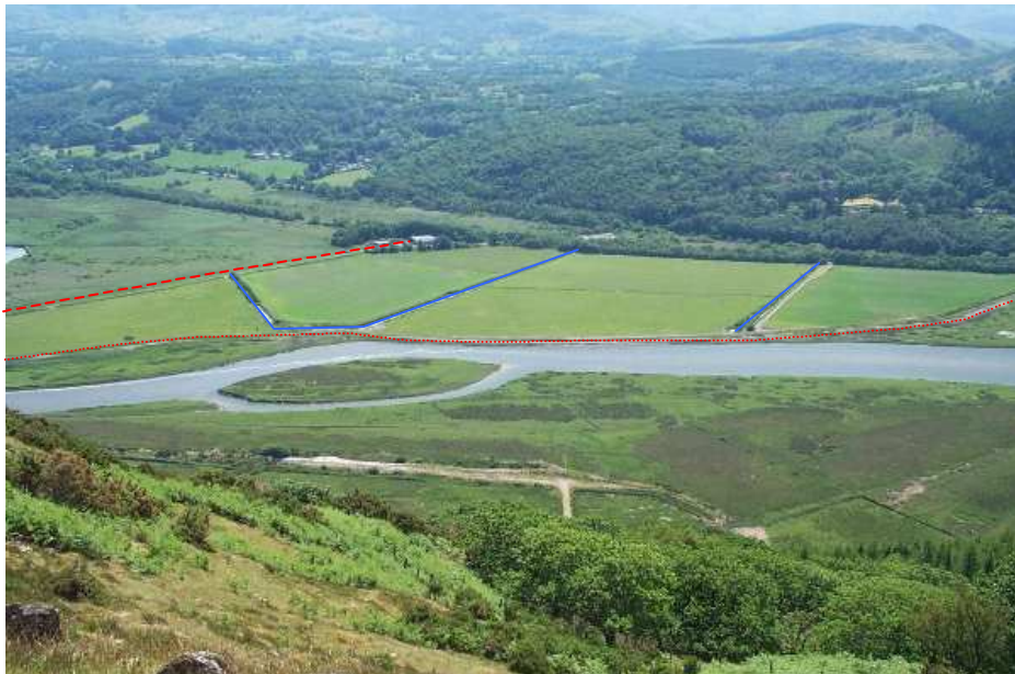
Figure 1.9: Land reclamation at the head of the Mawddach estuary. Earth embankments are marked in red, and drainage ditches in blue.
